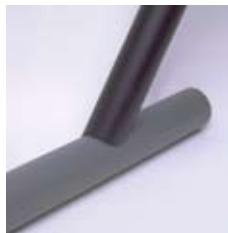
Step 4: Ready to weld
